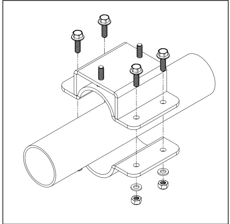
2. Using the supplied M6 hardware, attach the crossbar bracket over the chosen aftermarket crossbar. Tighten until crossbars are secure.
